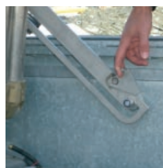
4. Support for lid with safety ratchet.
